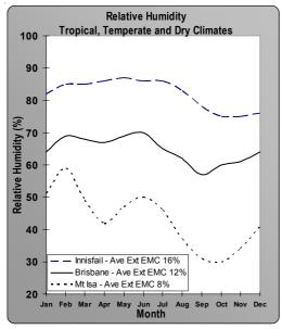
Figure 1 Climatic effects on timber floors
