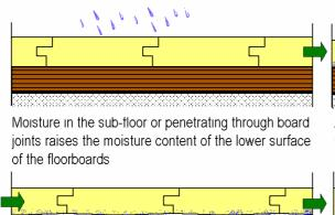
The floor is sanded flat, but higher moisture is still present in the lower surface of the board
