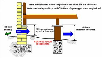
Figure 1 - Sub-floor Ventilation
