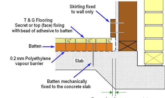
Figure 4 - Details of fixing in battens
