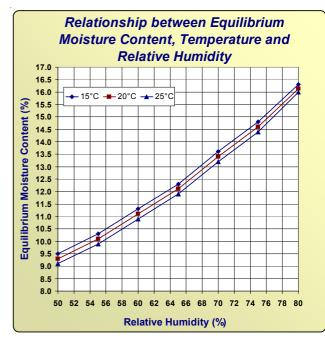
Figure 3 Temperature, RH and EMC
